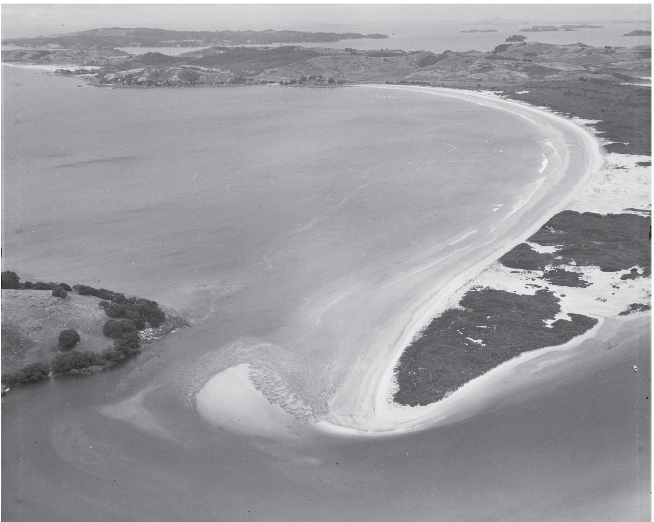
(Above): Aerial photograph of Omaha spit from 1953. A small sand bar can be seen to have formed where the ebb current leaving the harbour has met the littoral current flowing north along the beach. Compare this with the aerial photos from 1963 and 1976. Photo courtesy of Whites Aviation Collection (WA-32400), Alexander Turnbull Library, Wellington, N.Z.
